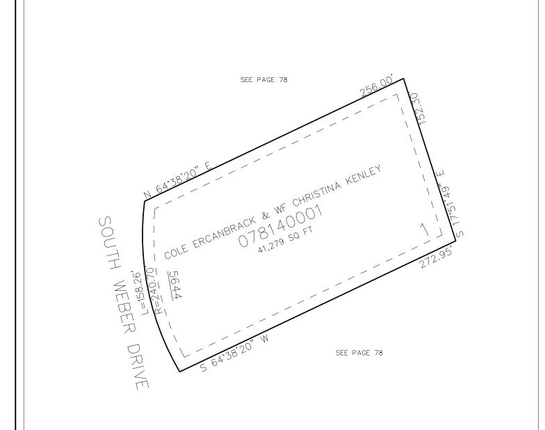
10' UTILITY & DRAINAGE EASEMENTS EACH SIDE OF PROPERTY LINES AS INDICATED BY DASHED LINES EXCEPT AS OTHERWISE SHOWN.
